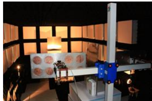
Figure 9 A plate type aluminum reflector target and CP antenna set-up inside the anechoic chamber.
