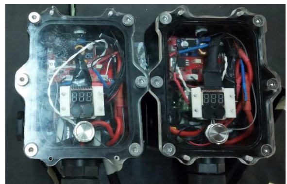
Fig. 5 Assembled control system with waterproof housing
