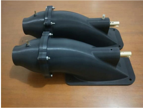
Fig. 9 Waterjet Propulsion for life buoy
